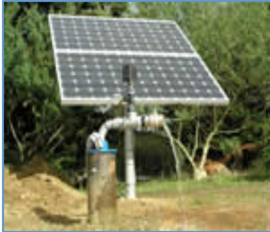
The big problem currently facing agriculture in reclaimed Egyptian desert far away from an electrical grid is dependence on diesel powered generators that require difficult to deliver and expensive liquid fuels for their operation. Off-grid<sup>1</sup> solar water pumps that recover underground water from deep wells for agricultural uses using solar energy applications serve the unique needs of Egyptians who live in desert landscapes.
